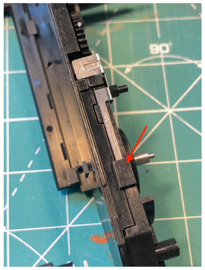
19. Now put back the counter wheel. The stud on the counter wheel must go through the loop of the torsion spring (shown in red circle), otherwise these two parts are not connected so the counter wheel won't reset automatically.
