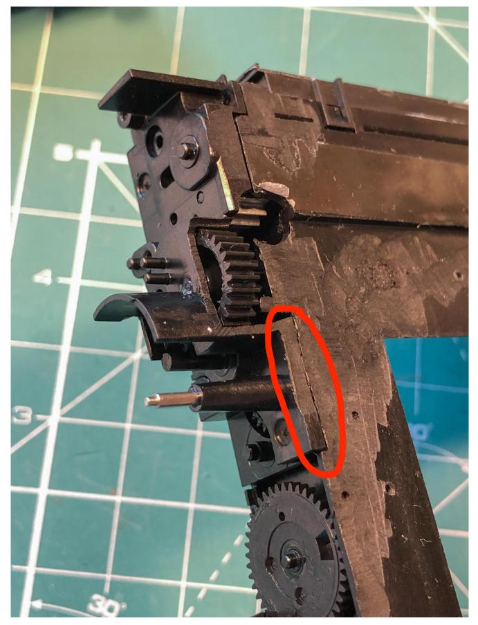
13. With the broken gear removed, rotate this gear with your finger again to see if everything's smooth. You shouldn't feel any resistance.
