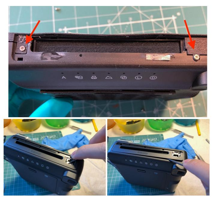
4. Now the back should come apart easily. We will only work on the ejection unit in the middle (red box) for now.
