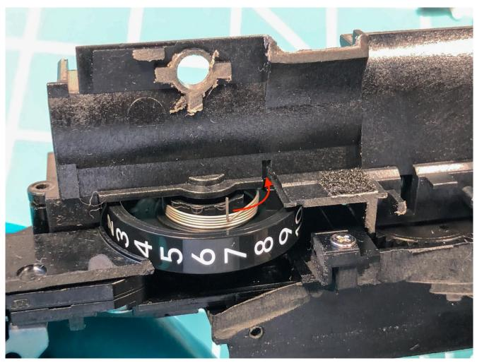
23. In this step, I separated the parts so you can clearly see what is going on underneath. Don't actually separate these, you've just put them back together!
