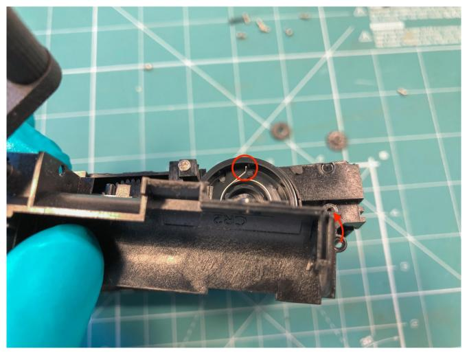
22. Looking from the other side, the bend of the spring must be in this groove when properly assembled.
