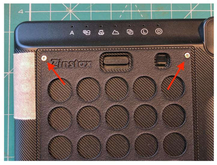
3. There are two more screws hidden under the top cover. The top cover is glued in place, you can pry it off with something pointy (a knife, I use an awl, fingernails work just fine too). I usually stick the awl under the cover to lift it up, and then slide the awl along the edge to break the bond.
